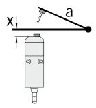
The axis of the hinge should be x mm above the top edge of the safety switch and in the same plane. a = Actuating radius to the plane of the actuator x = Axial misalignment
