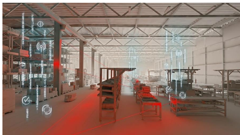
Fig. 3: Signals from wireless sensors at shop-floor level are received by Access Points and passed on to a Sensor Bridge
