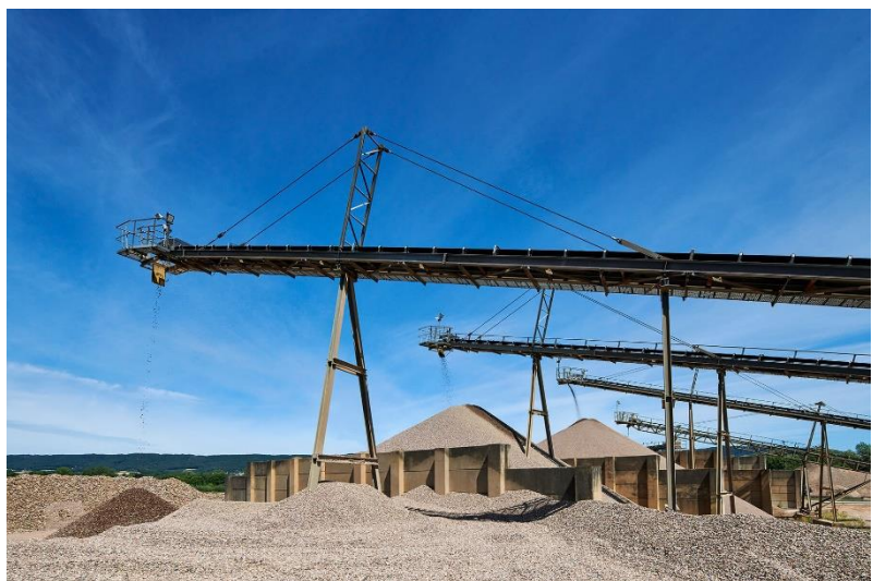
THE PLANT is designed for a throughput of up to 220 t/h. A load-dependent control system ensures energy-efficient grading.
