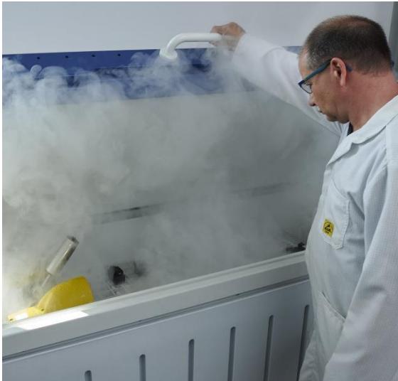
01 The corrosion resistance level of the switches is tested in a salt spray chamber
