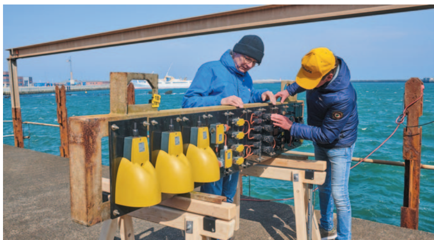
Deep dive and pressurizing: waterproof tests of foot switches in the steute lab (and, below, in situ).
